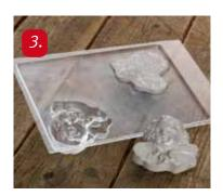
3. Let the concrete dry for at least 24 hrs, cover with a plastic sheet. Spray the concrete with water a couple of times when drying. Carefully remove the concrete from the mould when it is completely dry.
